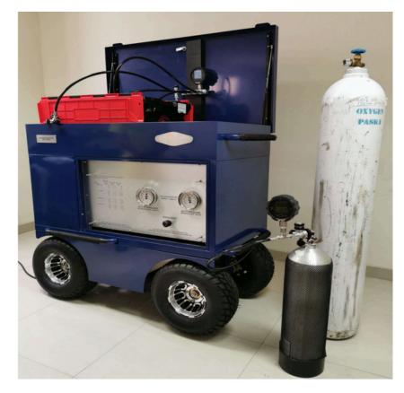
Booster is wheeled onto site, plugged into mains AC, the lid is opened and cylinders connected. The inlet is connected to a gas supply. Press the start sequence, and four cylinders are flled at the maximum safe rate for oxygen flling
