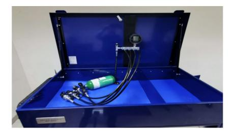
Booster lid accommodates dry filling as shown below on silicone pad, or an 80L HDPE wet tank (supplied and seen in the image above). One to four cylinders are filled simultaneously.
